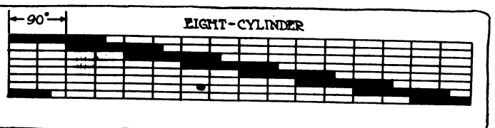
Fig. 17—Chart of overlapping power impulses for an eight drawn in the same way as Fig. 18
